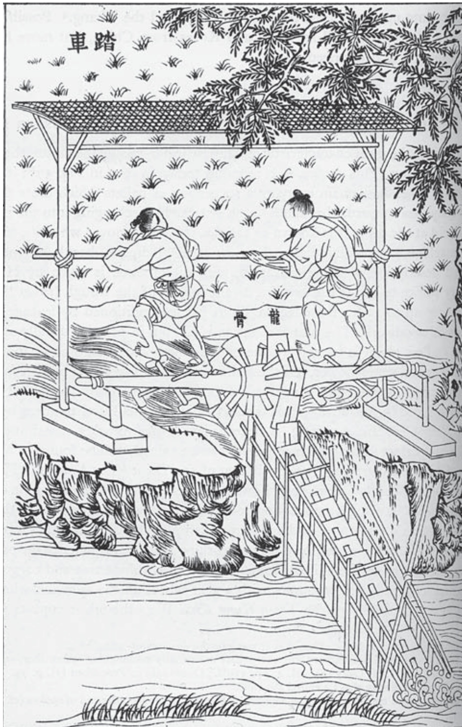
The square-pallet chain-pump, a Chinese water-raising machine, as pictured in the Thien Kung Kai Wu ( The Exploitation of the Works of Nature ), a book published in 1637.
